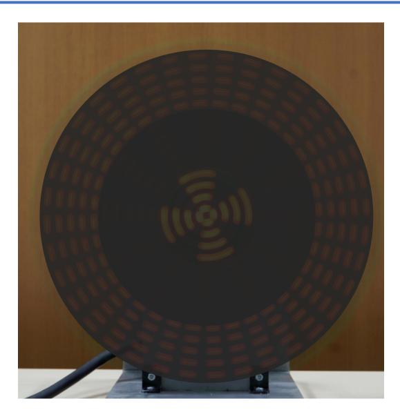
Outside zone High-density light trails for high-capacity transmission
